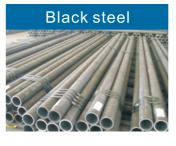
Black steel is a term given to steel pipe with a black oxide scale on the surface. This black oxide scale is formed when the pipe is forged and is typically sealed with a protective oil to prevent corrosion. Because of this oxide scale and protective film, black steel pipe requires little maintenance and is used for a wide variety of applications, including in water, steam, air and gas services.
